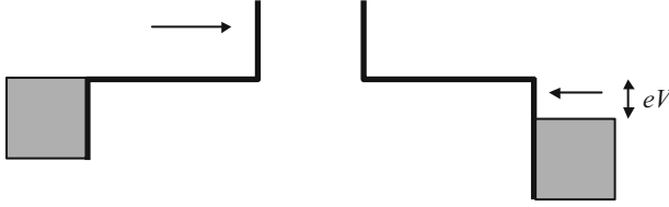
Fig. 16.3 Illustration showing the assumption that the charge reservoir on the right is shifted down by eV and that the electric field is not affecting the band structure of the system
