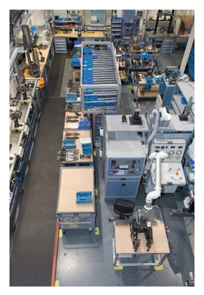
Fig. 10.6 Product—flow layout/assembly line for refurbishment processes [front view] (© Knorr-Bremse Berlin SfS GmbH)
