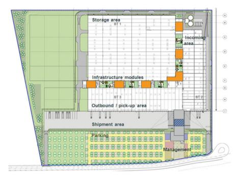
Fig. 10.11 L-shaped layout of a warehouse
