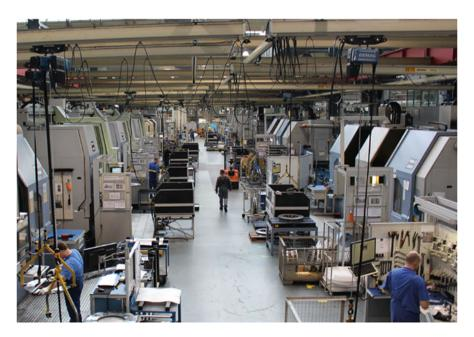
Fig. 10.4 Machine-centers for turning, milling, and drilling (C Knorr-Bremse Berlin SfS GmbH)
